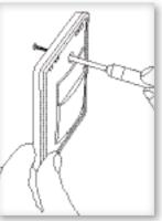
Insert the trim plate tabs into the bottom slots of the key card switch, and then lightly flex the trim plate to insert the top tabs.
