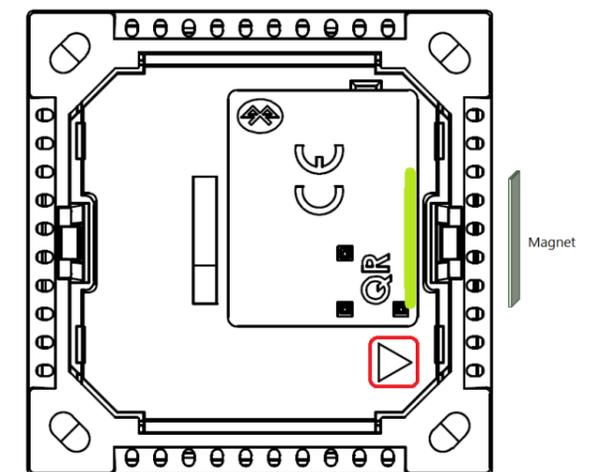
Attach the magnet to the intended surface (e.g. door or window) so that it aligns with the center of this side and verify that the distance between magnet and sensor housing is less than 1 cm (0.4"). Verify that the state (e.g. door open or closed) is reported as expected.
