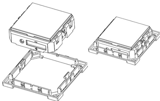
Note that backup battery and LRN button are protected from access after module installation into wall mount.
