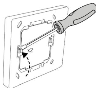
If necessary, the module can also be extracted from the front side without removing the wall mount from its installation location. To do so, carefully insert the screwdriver from the front between snap hook and module, press the hook outwards and lift out the module.
