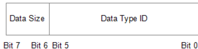
Figure 28 – Sensor Data Descriptor field structure
