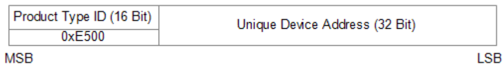
Figure 23 – BLE static source address structure
