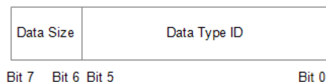
Figure 29 – Sensor Data Descriptor field structure
