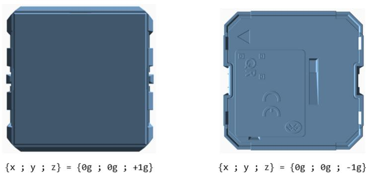
**Figure 62 – Acceleration vector based on device orientation**
