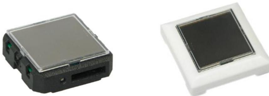
**Figure 1 – STM 550 module (left) and finished product (right)**
