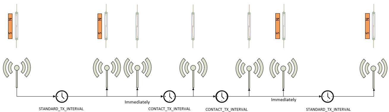
**Figure 7 – Magnet contact sensor-controlled reporting interval**
