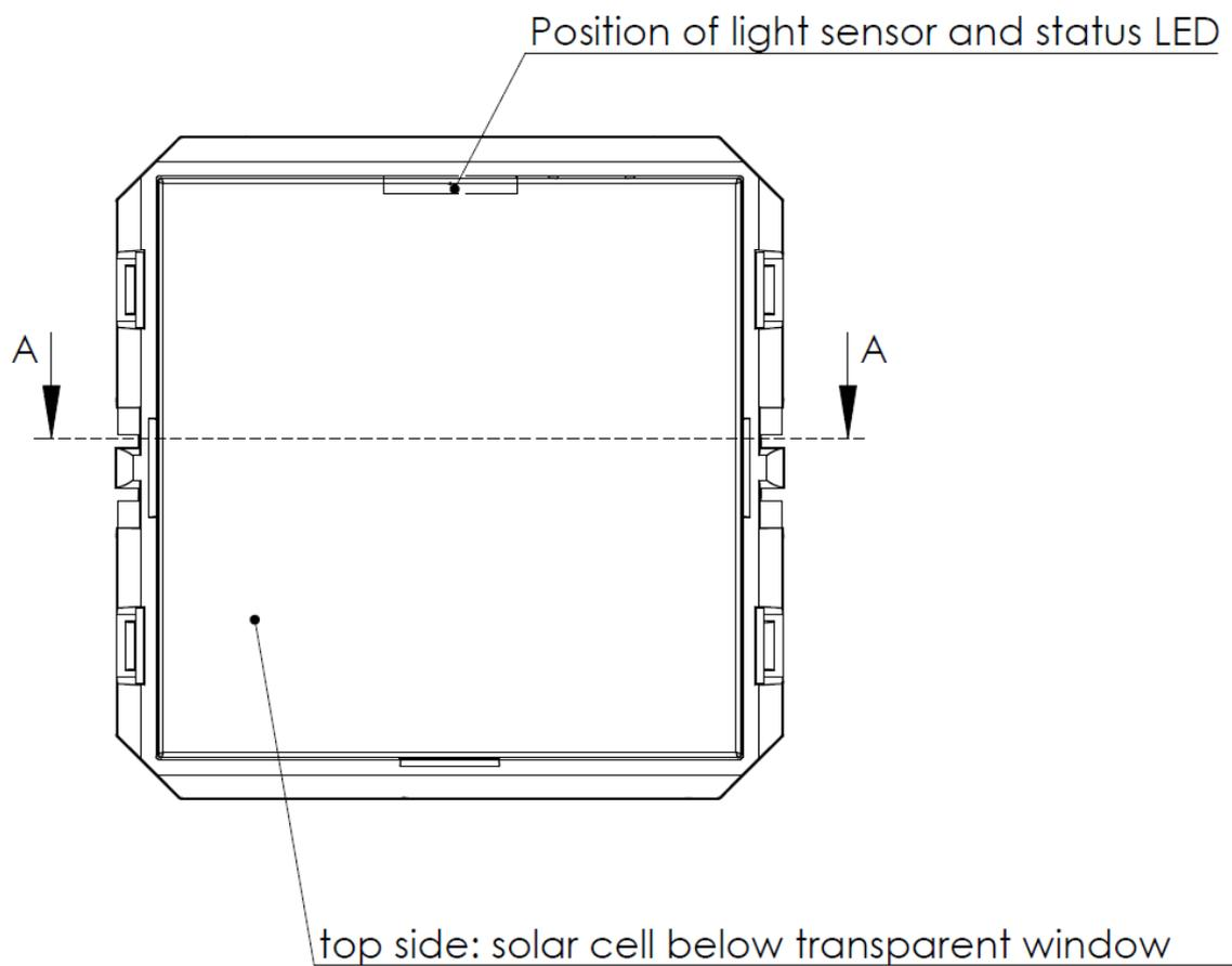
**Figure 56 – Top view of STM 550 module**
