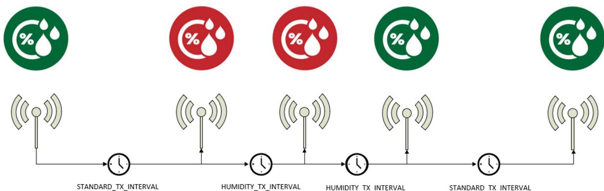
**Figure 5 – Humidity-controlled reporting interval**
