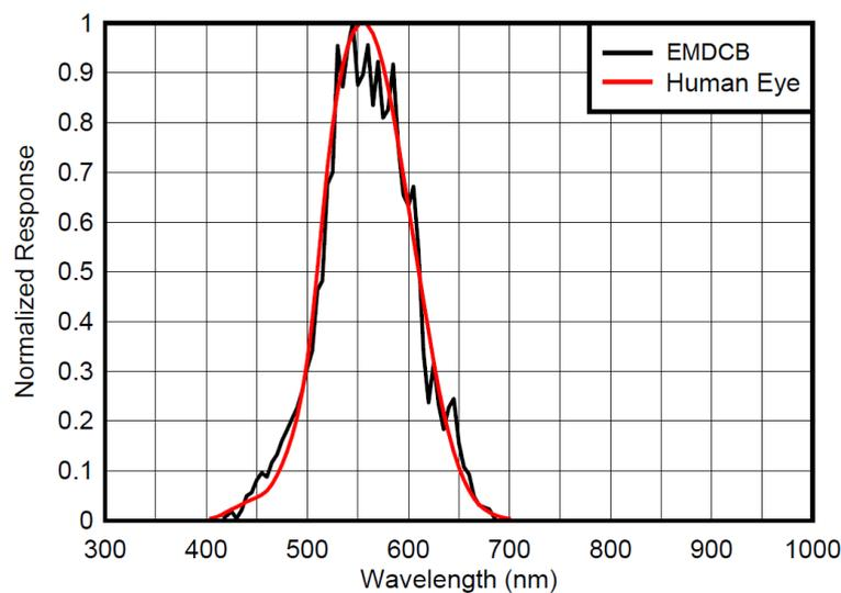
**Figure 8 – Spectrum response of the light level sensor**
