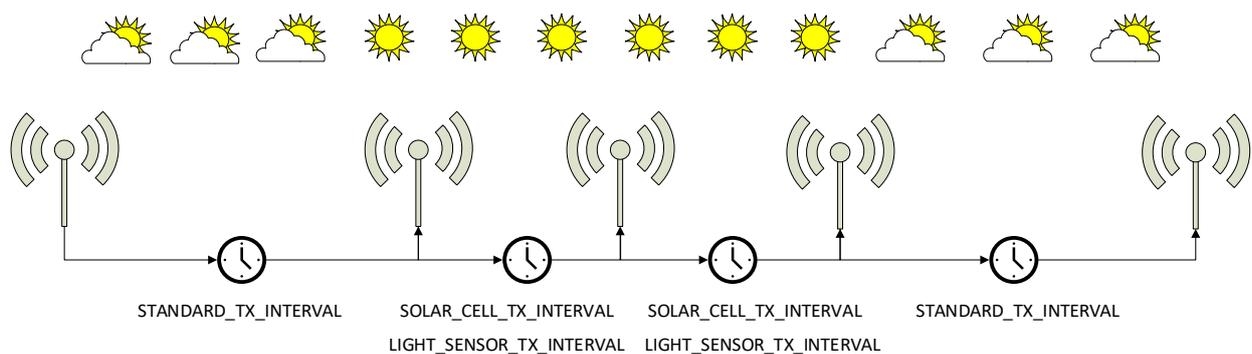
**Figure 3 – Illumination-controlled reporting interval**
