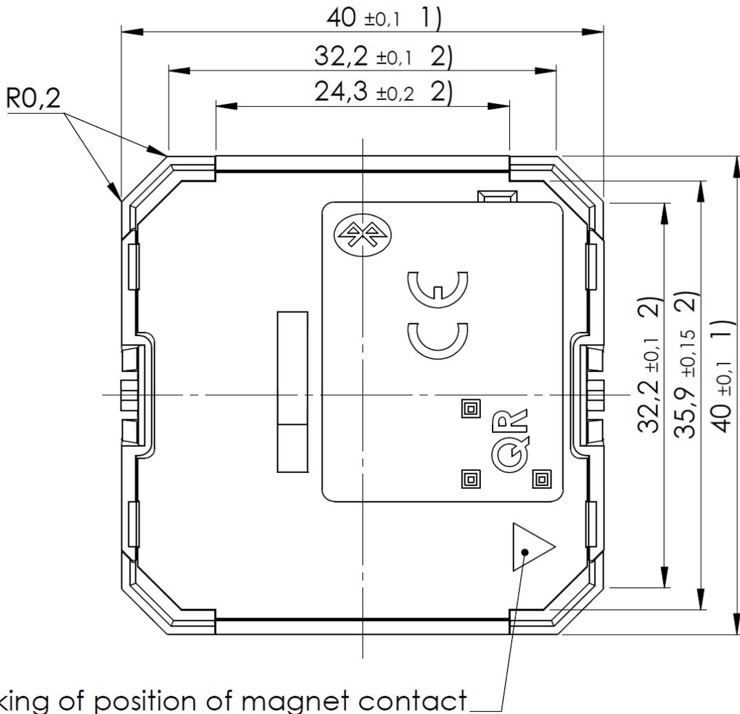
**Figure 57 – Bottom view of STM 550 module**
