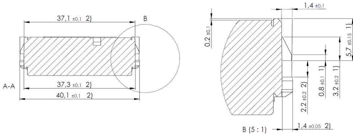
**Figure 58 – Cut view (A-A) of STM 550 module**
