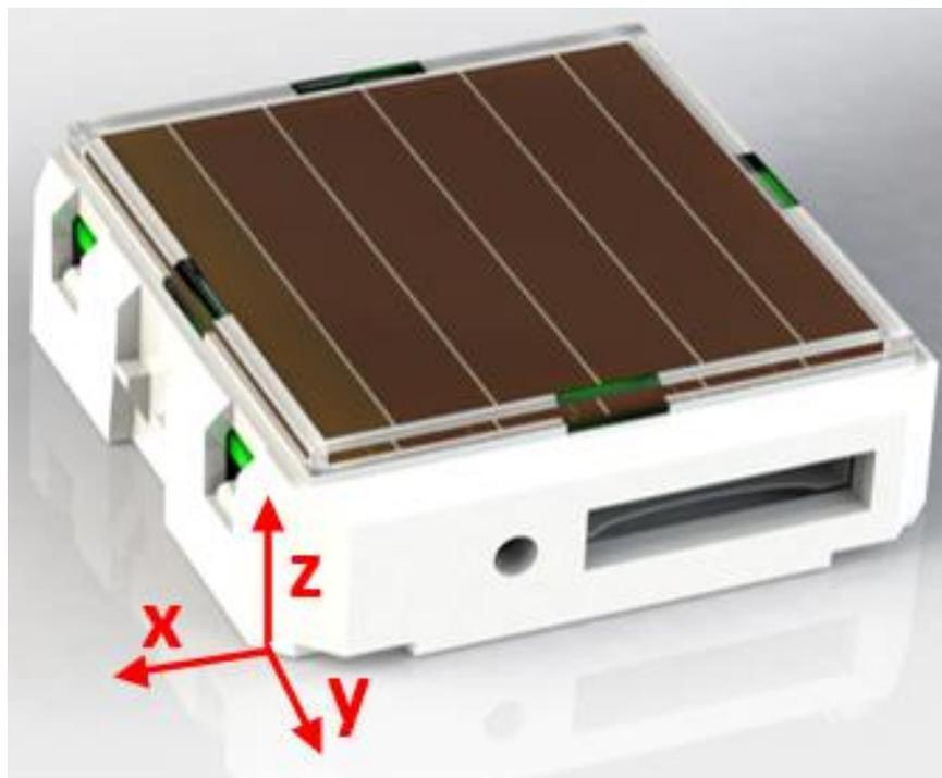
**Figure 11 – Acceleration sensor orientation**
