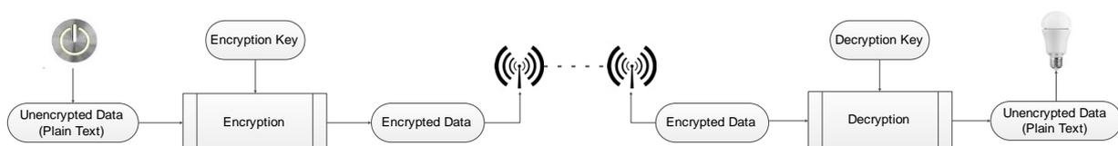
**Figure 22 – Telegram encryption**
