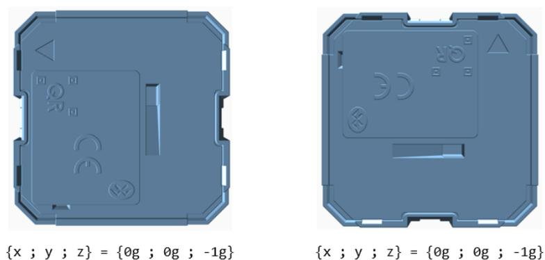
**Figure 63 – Device rotation across earth gravity vector axis**
