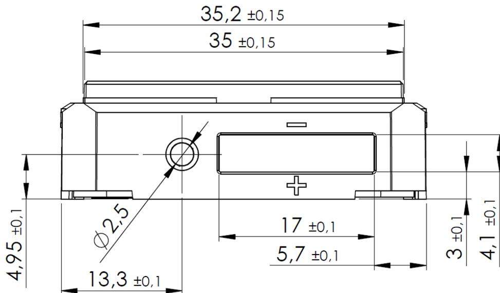
**Figure 59 – Front view of STM 550 module**
