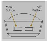
NOTE: The button interface on the sensor is used for linking and testing only. The occupancy timer settings are configured on the transceiver to which the sensor is linked.
